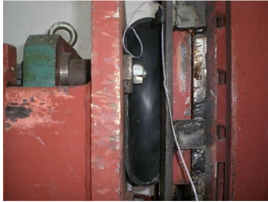
Partially deformed shape of the specimen
