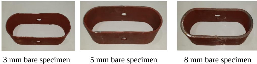
Figure 2.1 : Bare steel cushion samples.
