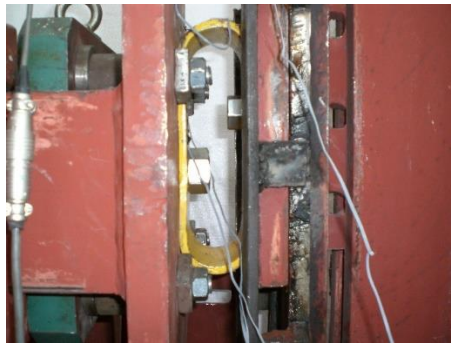
Partially deformed shape of the specimen
