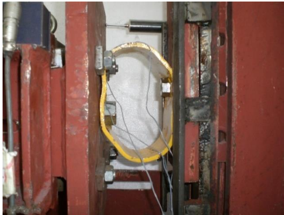
Partially deformed shape of the specimen
