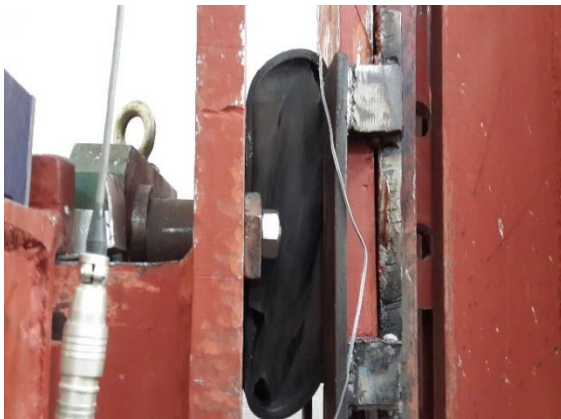
Partially deformed shape of the specimen
