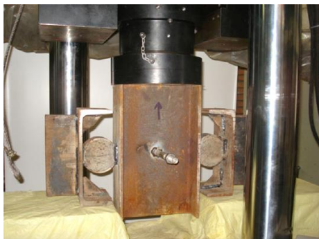
General view of the filled steel pipe under shear test
