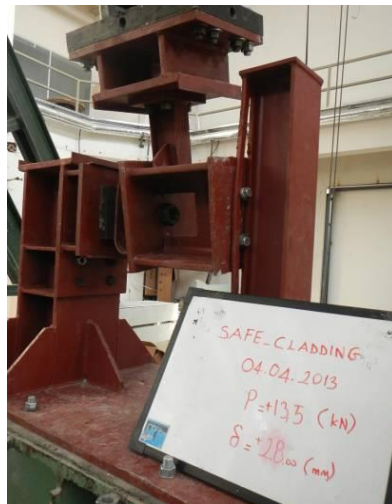
Figure 2.10 : Out of plain deformations in the setup.
