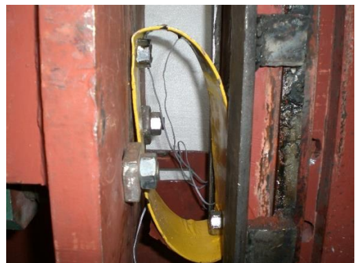
Ultimate deformed shape of the specimen
