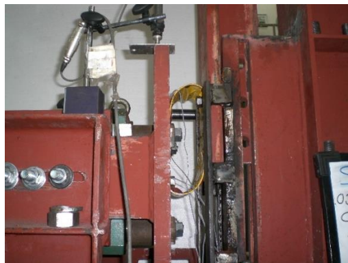
Ultimate deformed shape of the specimen
