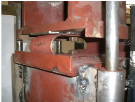
Partially deformed shape of the specimen
