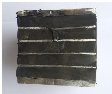
8 mm infilled steel layered specimen
