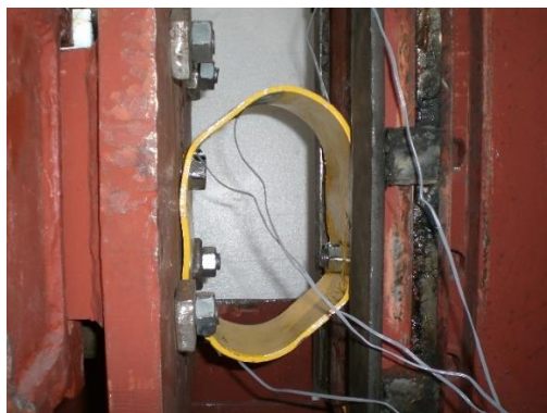
Partially deformed shape of the specimen
