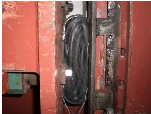
Partially deformed shape of the specimen
