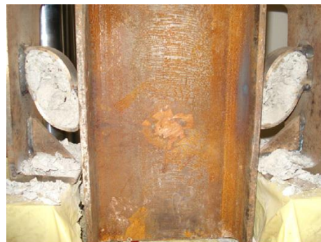
Typical deformed shape of filled steel pipe specimen
