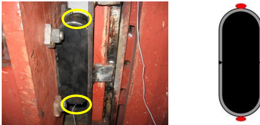
Figure 2.23 : Strain gauges on the outer top and outer bottom of the specimen.
