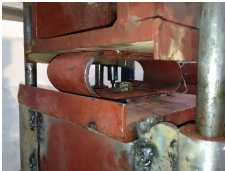
Partially deformed shape of the specimen
