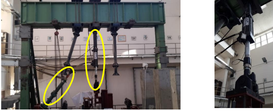
Figure 2.5 : Actuator holder system with the related actuators and closer view of the actuator.
