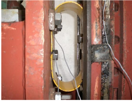
Partially deformed shape of the specimen
