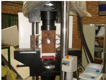
General view of the bare steel pipe under shear test
