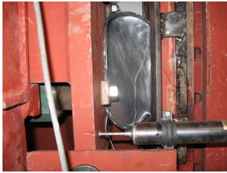
Partially deformed shape of the specimen
