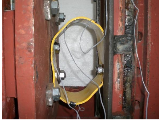
Partially deformed shape of the specimen
