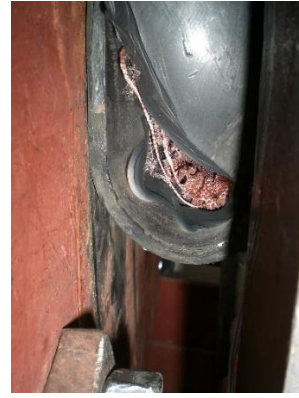
Ultimate deformed shape of the specimen
