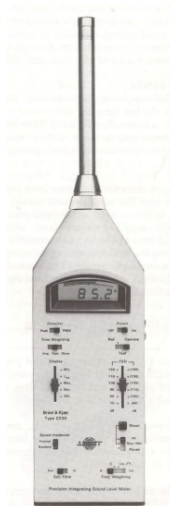
Figure 6.3. B&K Sound Level Meter Type 2230 (Bruek & Kjaer, BB1078-14, 2003).
