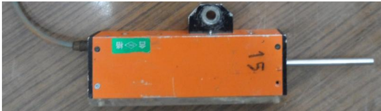
Resim 3.4. LVDT (Linear variable differential transformer)
