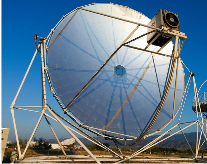
Figure 2.14 Solar dish concentrator (Günther & Shahbazfar, 2011)
