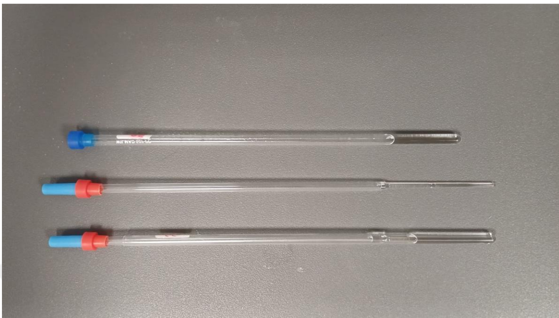
Figure 20: NMR samples with tubes and coaxial insert tubes. The main aim is to eliminate effect of reference molecule (DSS), so NMR reference tube is inserted separate tube with same paramagnetic properties.
