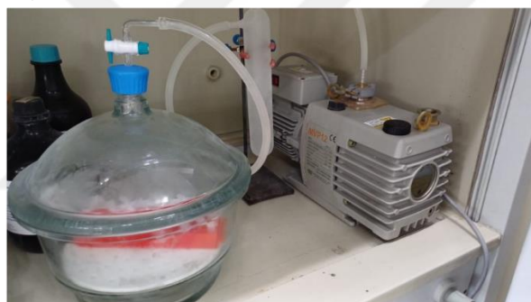
Figure 17: Lyophilization process of polymer solutions. Samples are frozen-dried by liquid nitrogen before they are transferred to desiccator. A) Samples are capped with an extra lid with three small holes to ensure water evaporation. B) Desiccator system connected to vacuum; samples are waited for at least 24 hours.
