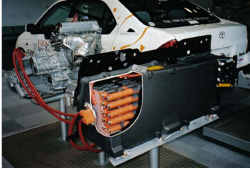
Figure 2.7. Nickel-metal-hydride battery of a Toyota hybrid car
