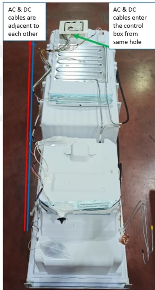
Figure 23: AC & DC cables entangled on the body and control box
