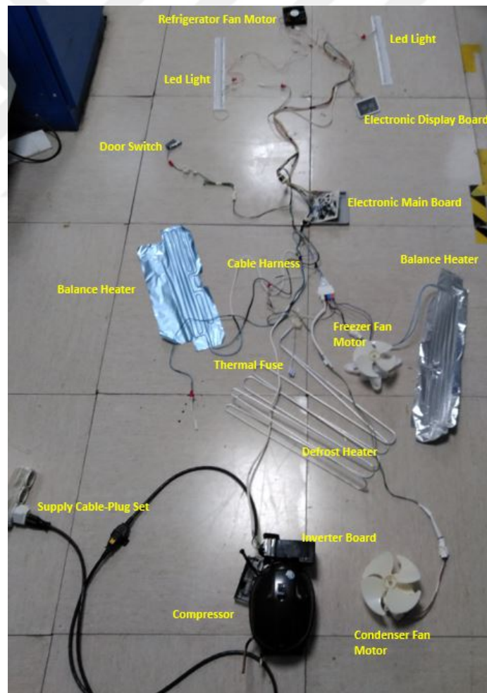
Figure 16: Main electrical and electronic components of a refrigerator
