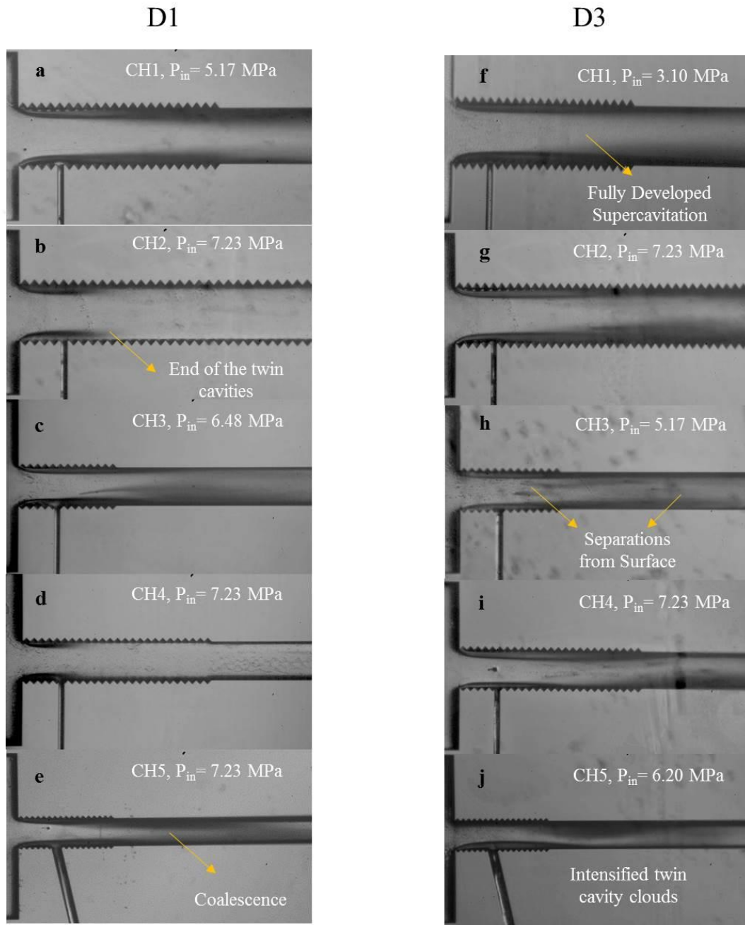
Figure 3-7 The comparison in the supercavitation flow regime inside different microchannels for the D3 coating with plain D1 microchannels
