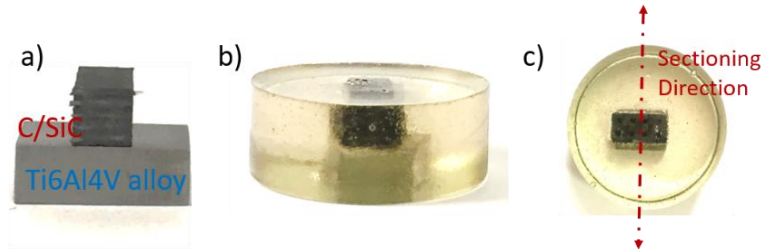
Figure 3.4 a) C/SiC composite-Ti6Al4V alloy joint sectioned into two types of specimen sizes, b) Epoxy resin mounted brazed joints, c) Sectioning direction of the brazed joints.
