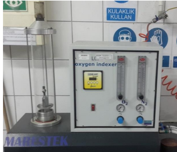
Figure 3.12 : Limiting oxygen index tester.
