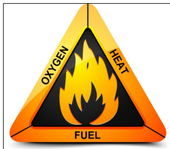
Figure 2.4 : Fire triangle of combustion [18].
