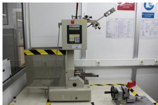
Figure 3.9 : Izod impact testing machine.
