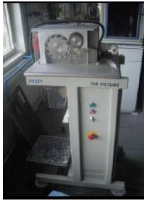
Figure 3.5 : Prism granulating unit.
