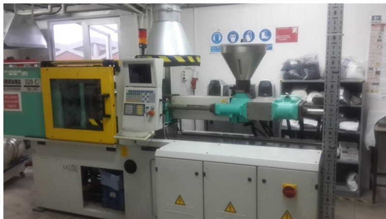
Figure 3.6 : Arburg Allrounder 320 °C injection machine.
