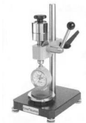
Figure 3.10 : Shore D Hardness test device.
