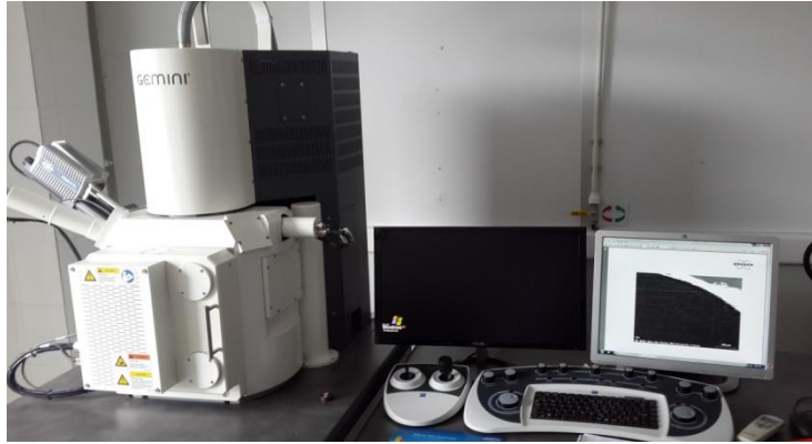
Figure 3.8 : Scanning electron microscopy (SEM).
