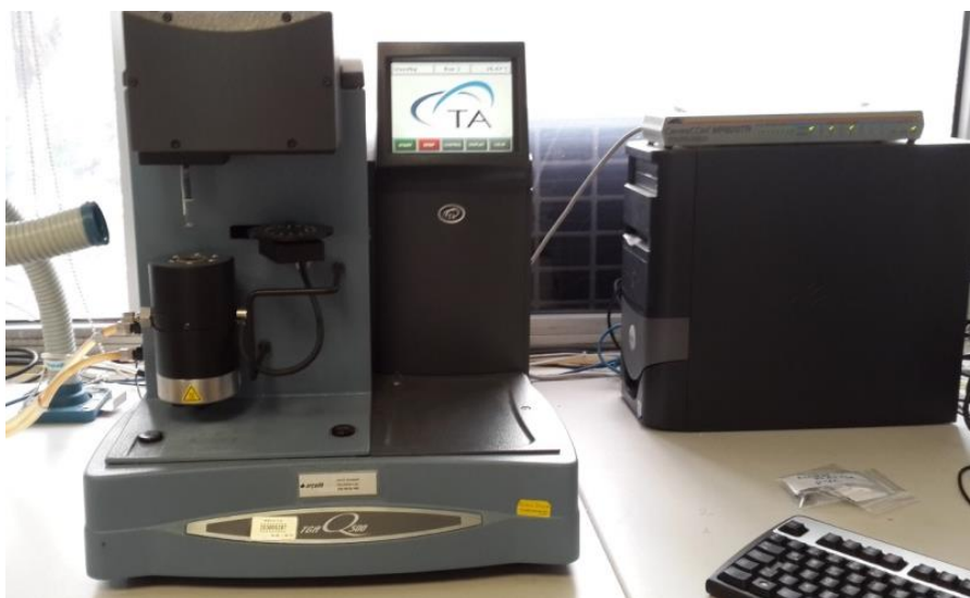
Figure 3.11 : Thermal gravimetric analyzer.
