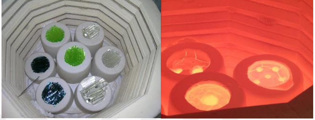
Görsel 3.9. Fırında Döküm, ( http://washingtonglass.blogspot.com/2010/10/boro-casting.html )
