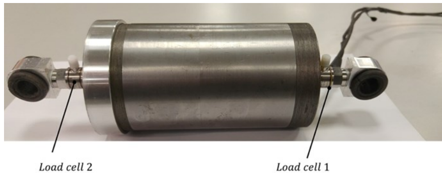
Figure 6.33: Load cells are utilized at two sides of 2 nd prototype of MR damper.
