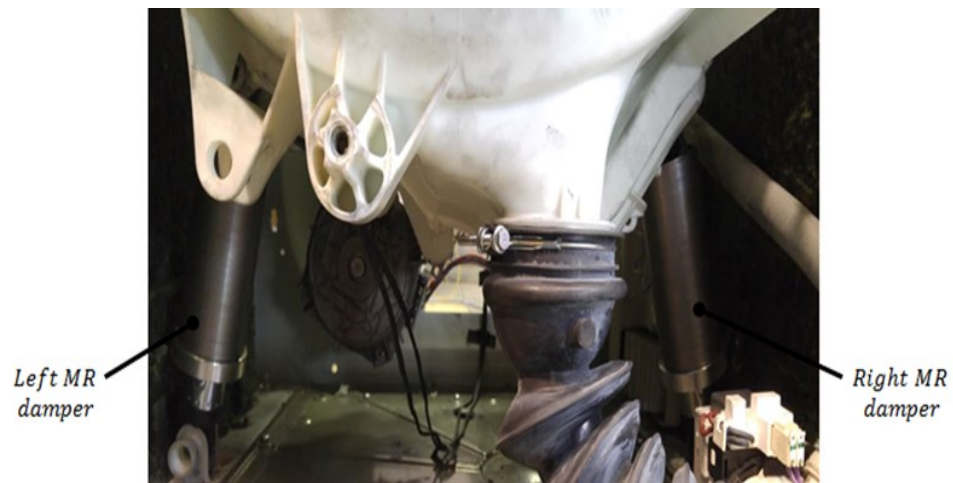
Figure 7.10: Two new 3 rd prototypes of MR dampers are used in washing machine.
