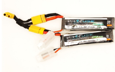
Figure 2.19: Two parallel 2S Li-Po batteries used to power the collision-resilient foldable drone
