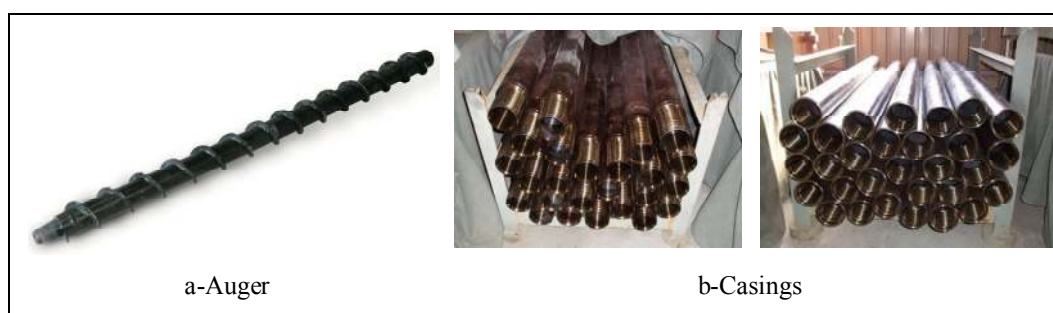
Figure 2.9 Some of the basic components of the auger type drilling tools.
