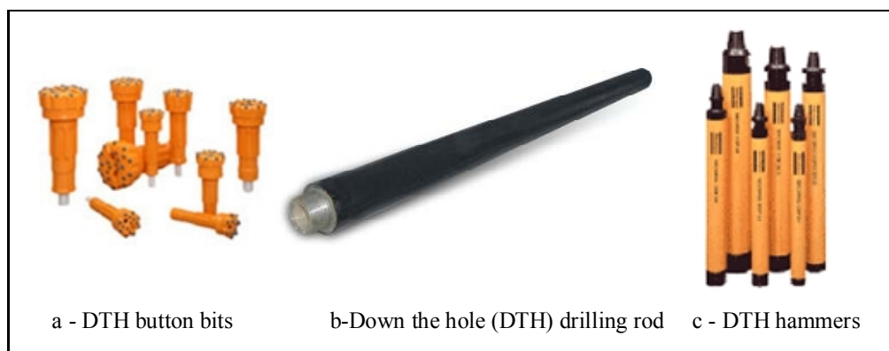
Figure 2.8 Some of the basic components of the DTH rotary-percussive type drilling tools.
