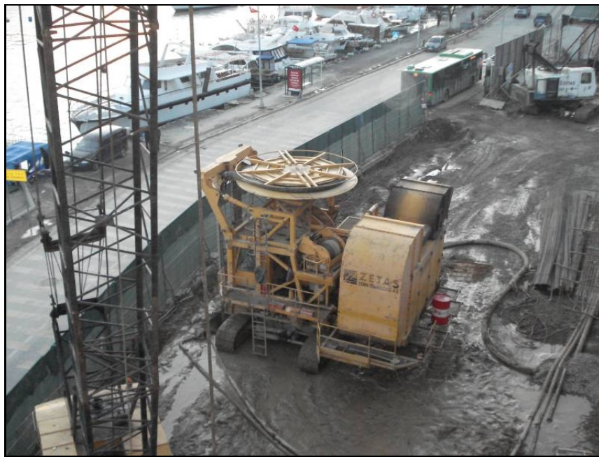
Figure 2.23 Compact hydraulic cutter - city cutter (Zetas, 2009).
