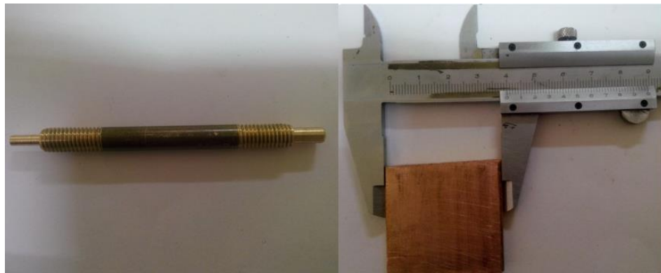
Figure 4.8 Brass tool and the copper workpiece
