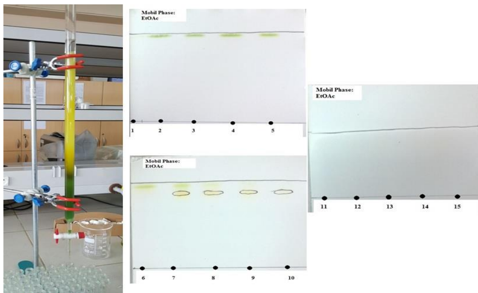
Figure 3.10 The column chromatography and TLC application of C. cylindracea extract (Personal archive, 2017)
