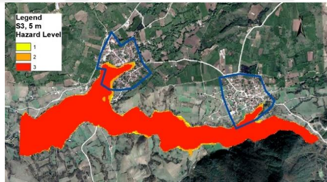
Figure 5-75 Flood hazard map for Avciidere Dam (S3)
