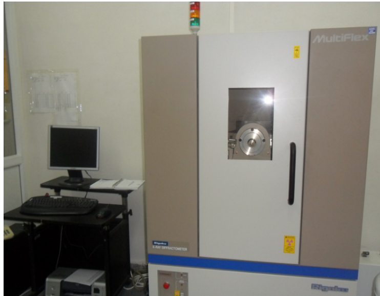
Figure 3.6: Rigaku X-Ray diffractometer
