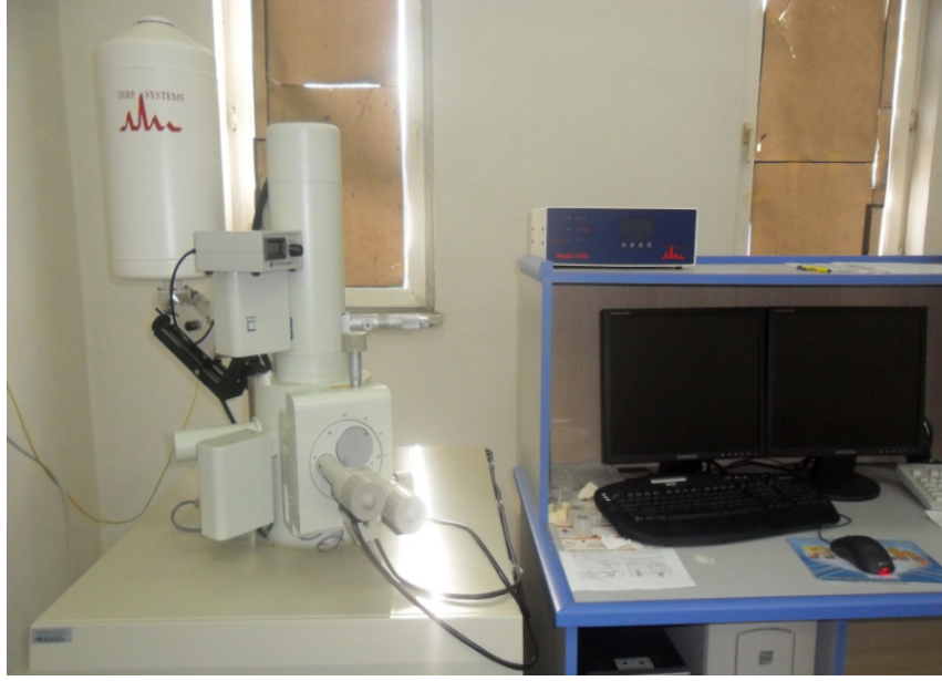
Figure 3.7: JEOL JSM-6390LV scanning electron microscope
