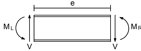
Figure 2.2. Free-body diagram of an isolated link segment
