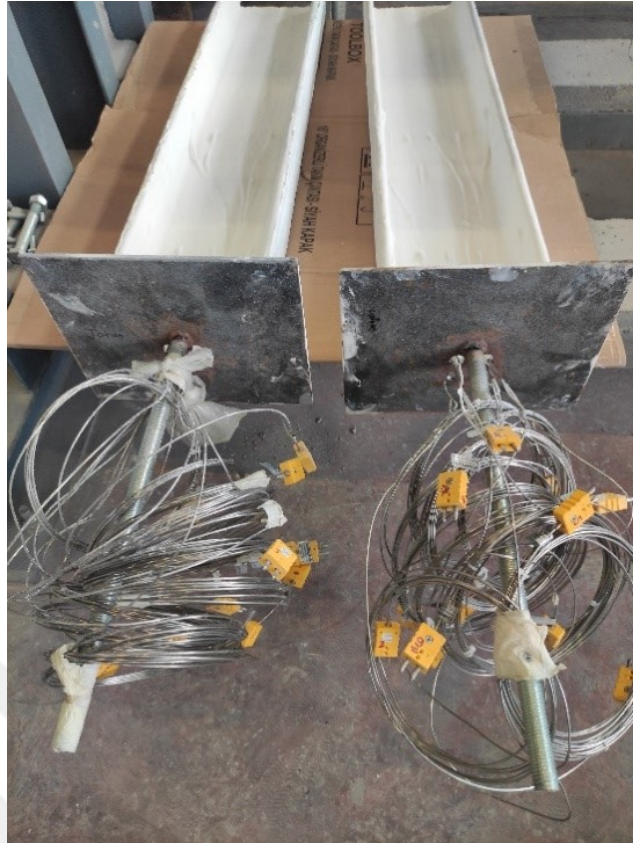
Figure 23: Specimens before the fire test after applying intumescent coatings.
