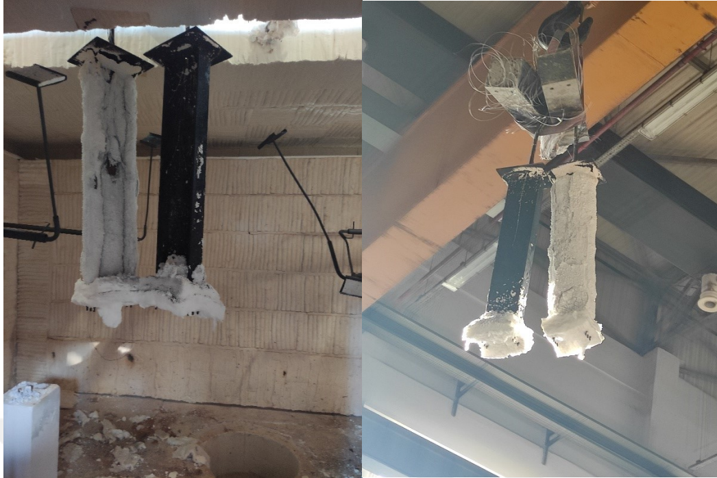
Figure 33: Specimens were removed from the furnace after the test to measure char thickness
