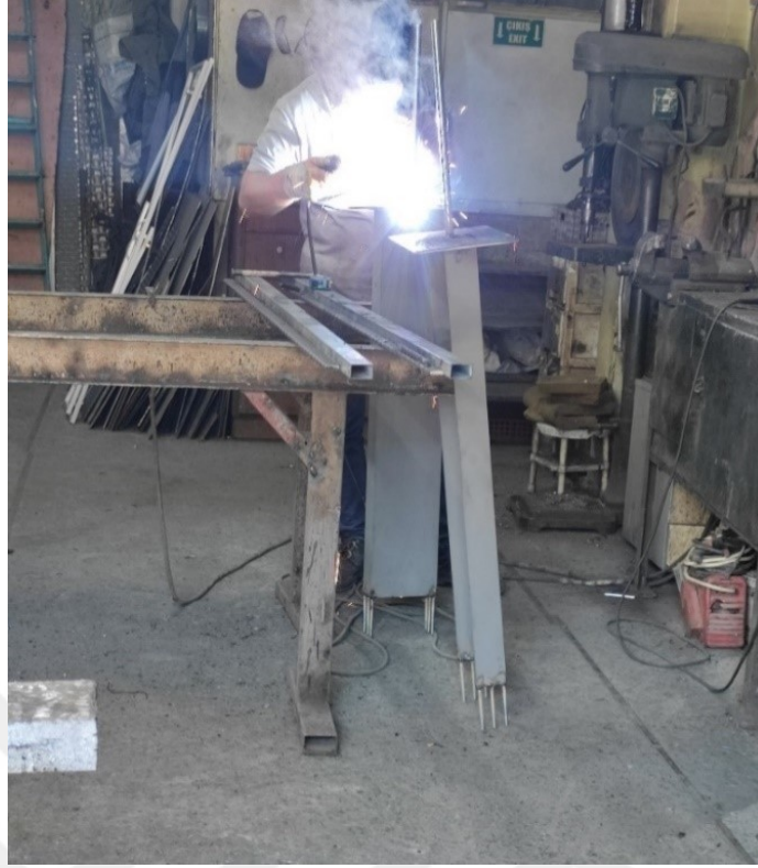
Figure 21: Welding the bolts to fix the beams in the furnace
