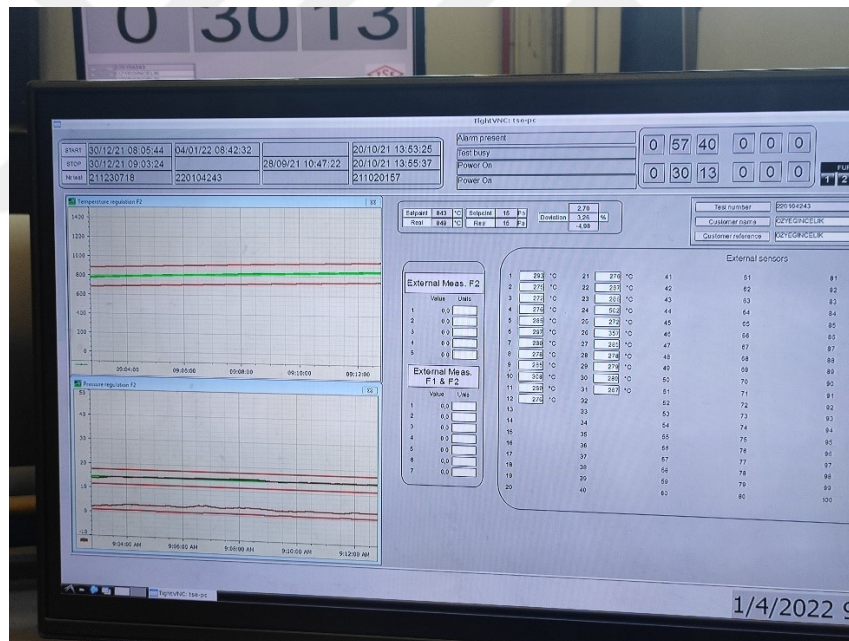
Figure 26: Thermocouples' initial values at the beginning of the experiment
