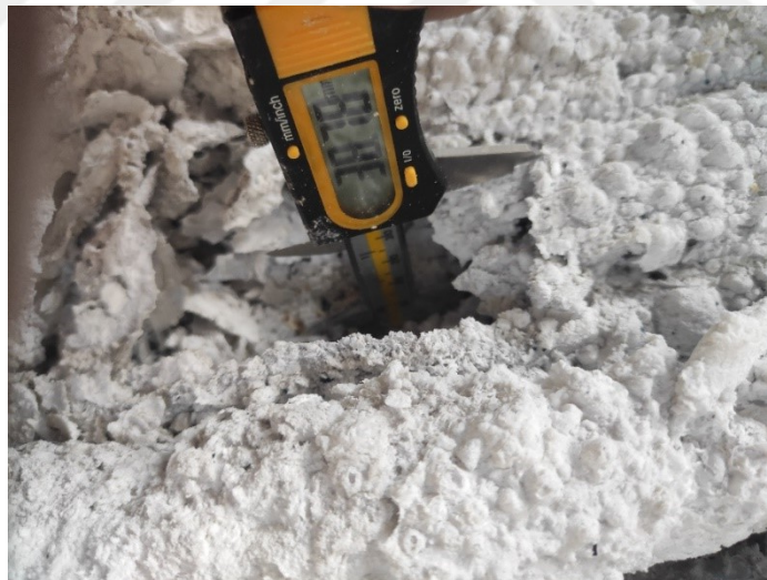
Figure 34: Char thickness for the Product A after fire test
