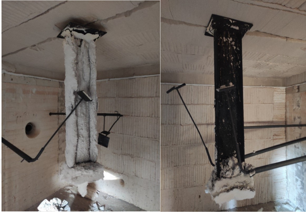
Figure 32: Specimens after the test, Product A is on the left and Product B is on the right
