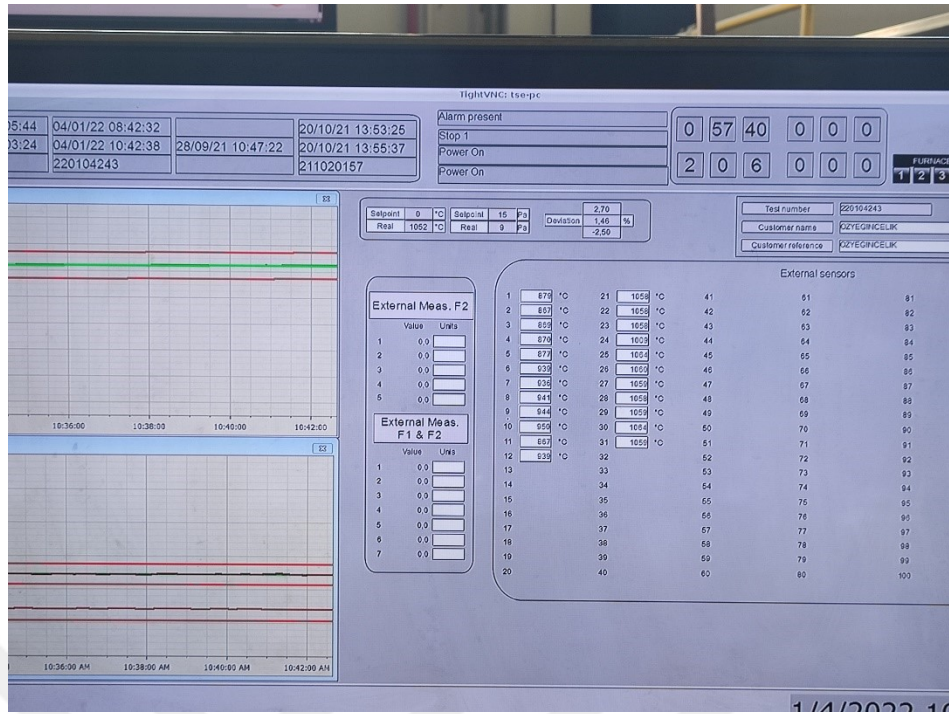
Figure 30: Thermocouple values of steel beams at the end of the experiment
