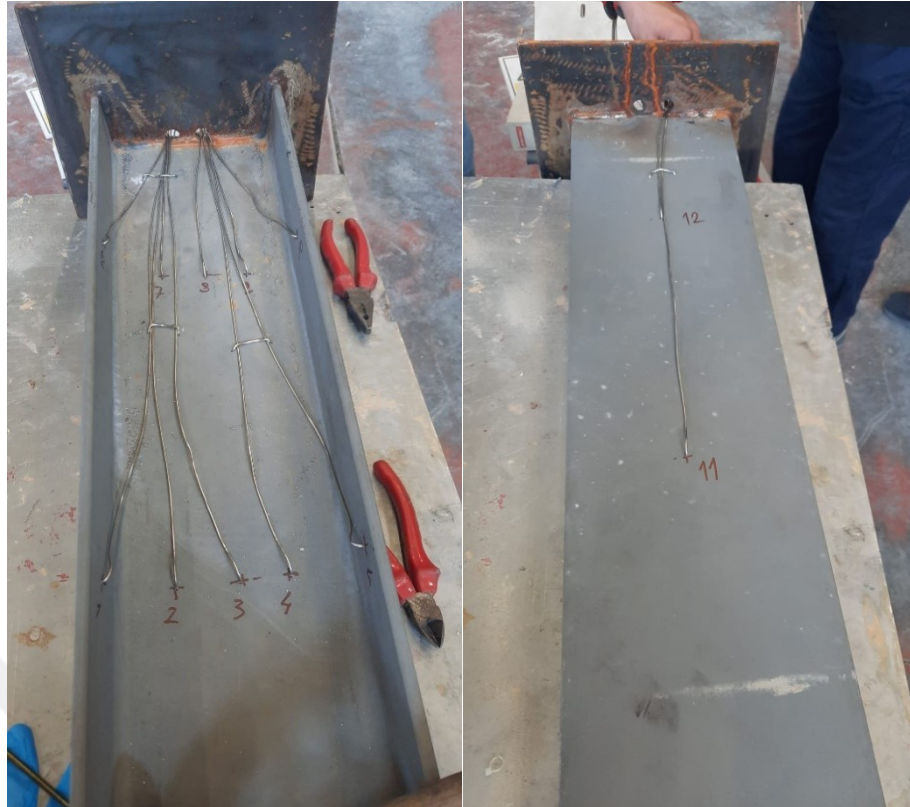
Figure 22: Fixed 12 thermocouples' locations for both Product A and B
