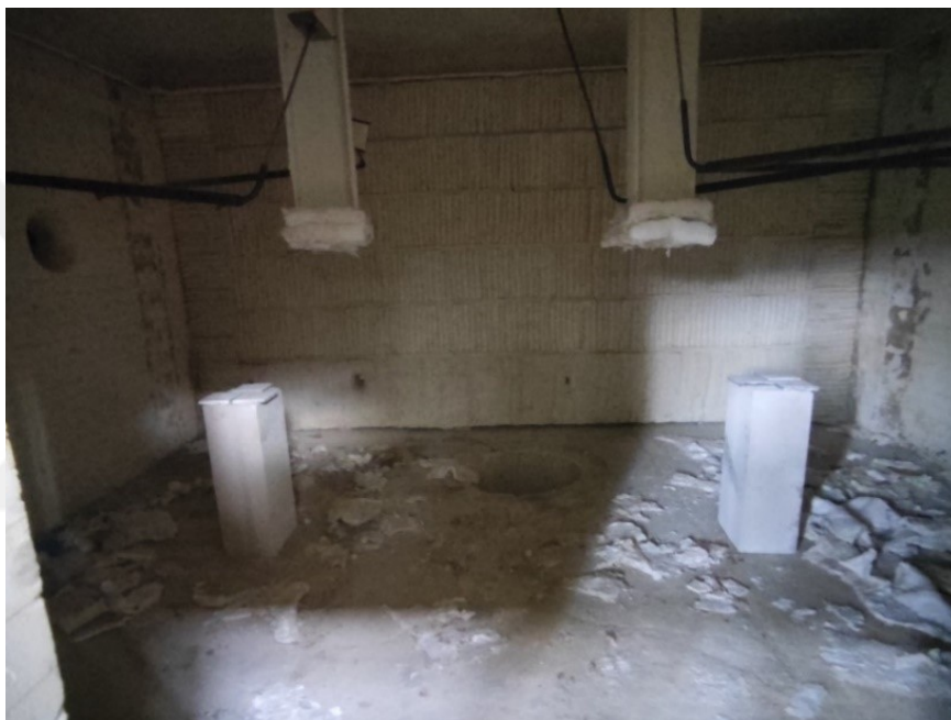
Figure 25: Specimens in the furnace just before the fire test
