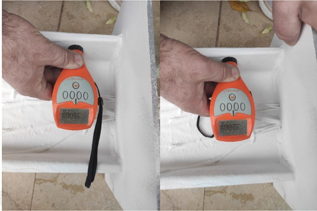
Figure 24: Measuring thickness of intumescent coating for Product A (on the left) and Product B (on the right)
