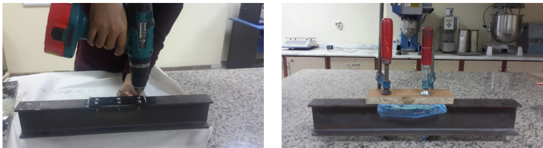
Figure 3.20. Employing bolts & clamping the specimens.
