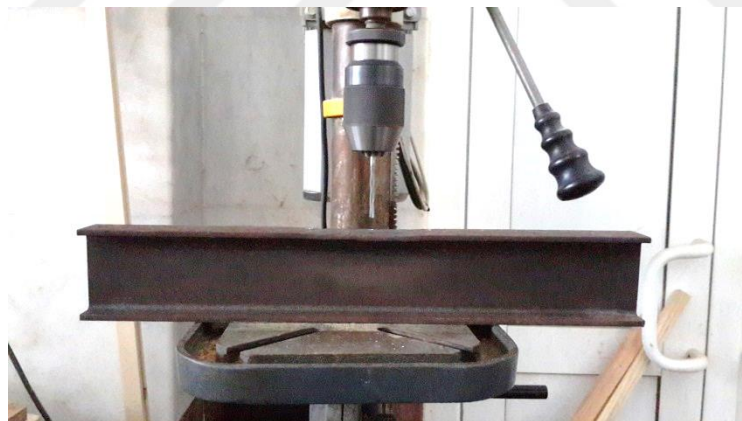
Figure 3.18. Drilling procedure for steel beam.
