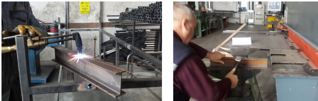
Figure 3.16. Heat treating and straightening of specimens.
