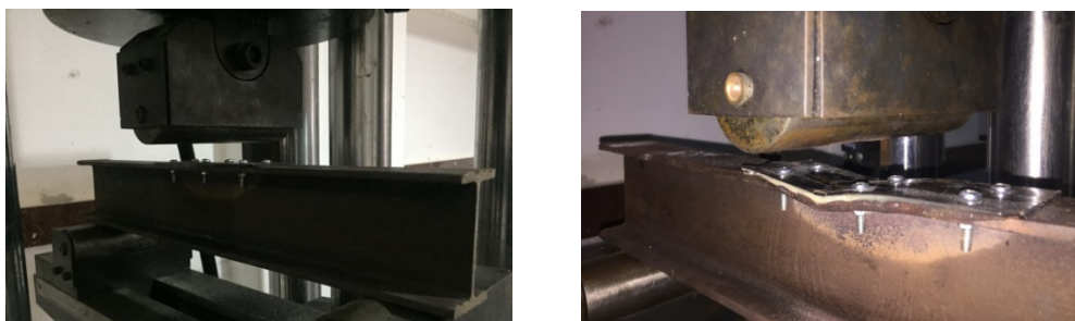
Figure 4.9. Retrofitted beams under three-point bending test.
