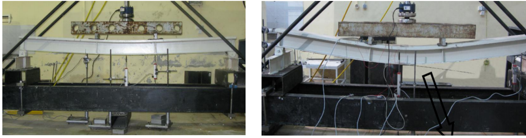
Figure 2.7. HM-CFRP strengthened composite I girder [32].
