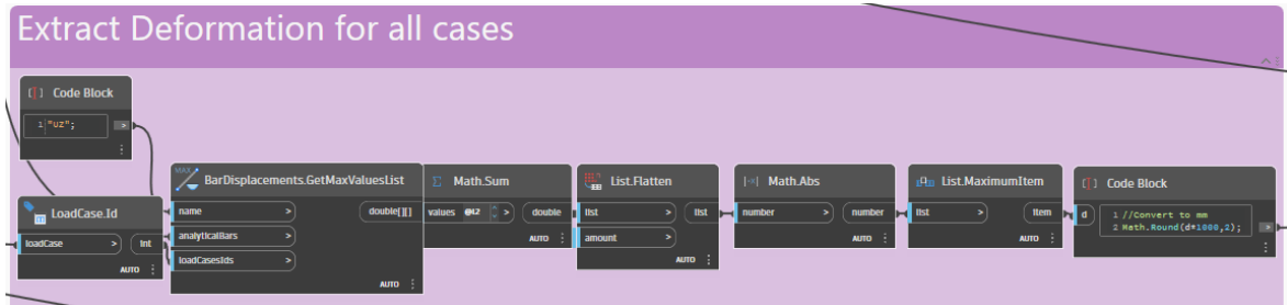
Figure 35. Extracting the deformations from the analysis
