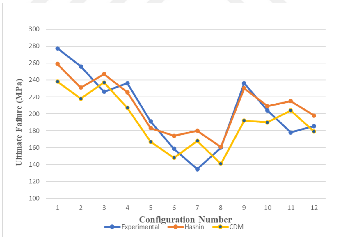
Figure 5.12. Experimental vs. MPDG vs. CDM damage evolution methods for all configurations of T300/1034C.
