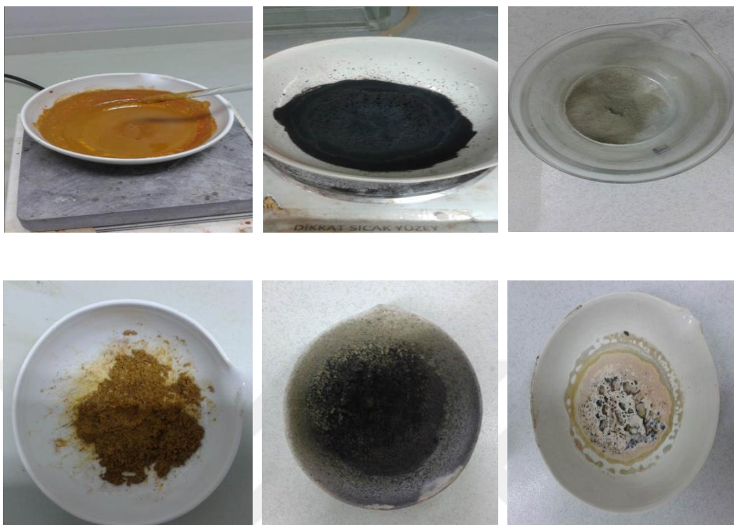
Picture 3.1. The examples of precursor gels and as-prepared products of vanadate compounds
