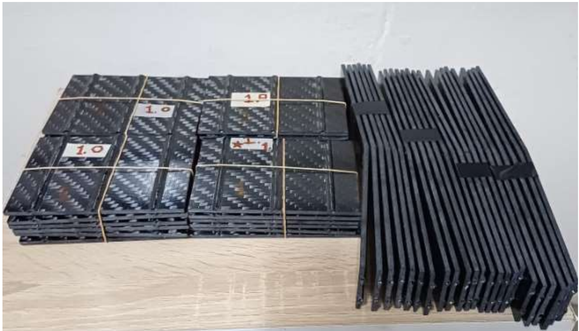
Figure 3.19. Prepared CFRP test specimens after cutting and classification according to test type (impact and bending )
