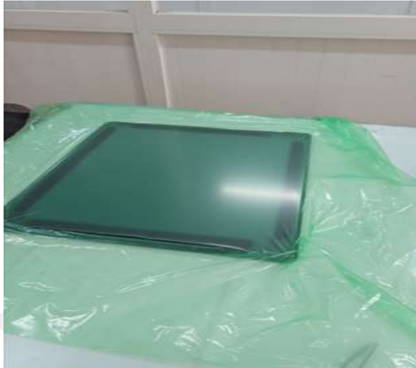
Figure 3.8. Nylon-based separation film applied to the MDF mould surface
