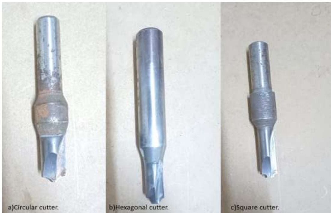
Figure 3.2. Profile cutters used for machining channels on surface of the molds: (a) circular, (b) hexagonal, and (c) square. All cutters are made of solid carbide material, selected for their high hardness and wear resistance during mold machining
