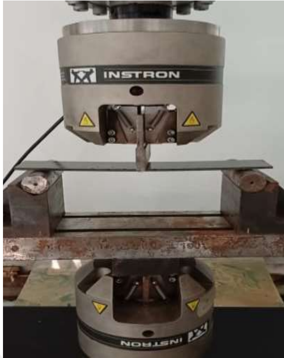
Figure 3.23. Three-point bending test setup used for bending testing of CFRP laminates (ASTM D790)
