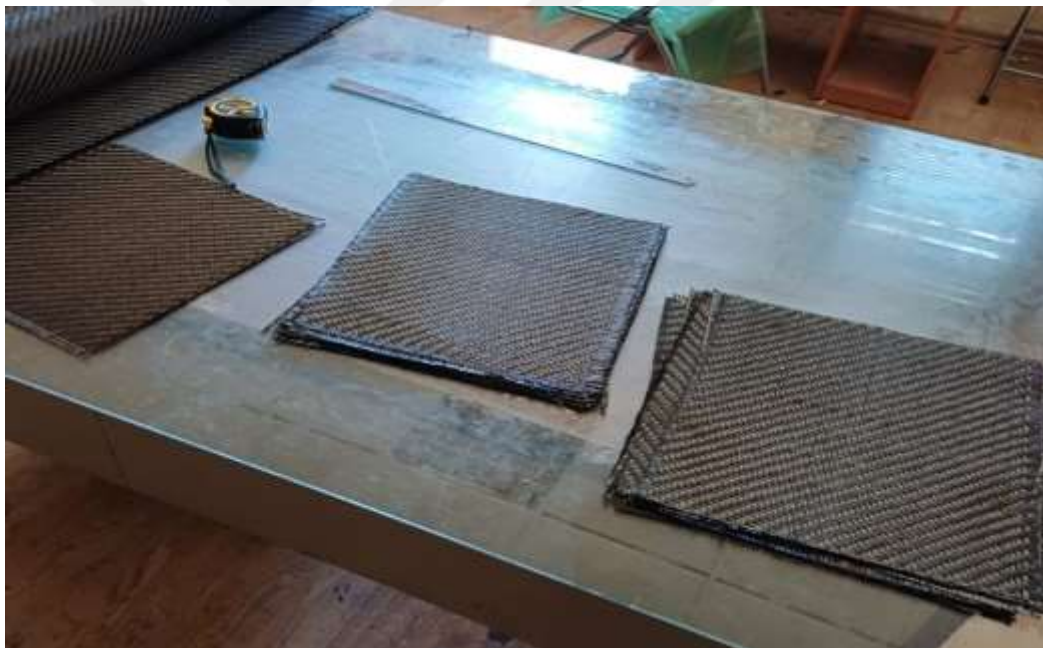
Figure 3.7. Preparation of twill carbon fabric layers for impact and bending laminates
