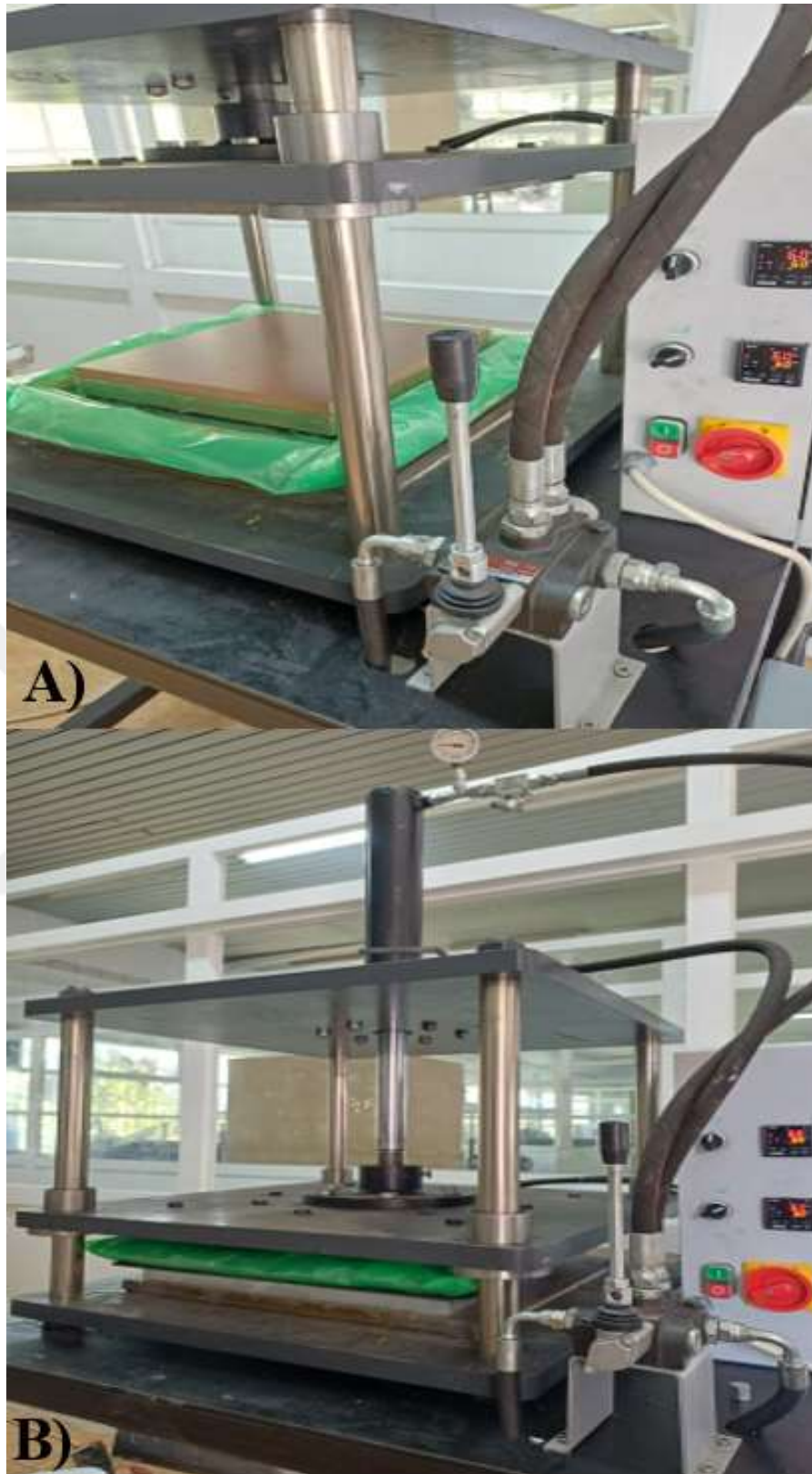
Figure 3.12. Curing process of CFRP laminates under hot press. (A) Placement of the prepared laminate between heated press plates prior to curing. (B) Curing process performed by applying hydraulic pressure and temperature in a laboratory-type hot press device
