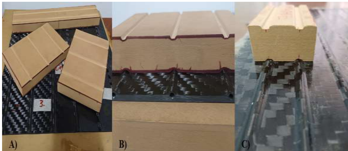
Figure 3.17. (A) Cutting templates for the bending and impact laminates produced, (B) Placing the cutting template prepared for cutting impact samples on the laminate in order to draw the cutting line, (C) Placing the cutting template prepared for cutting bending samples on the laminate in order to draw the cutting line.
