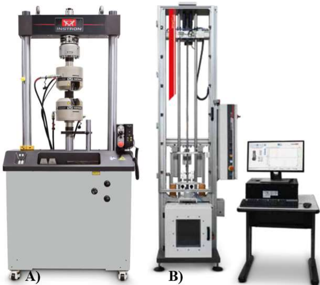
Figure 3.22. Test equipment used for mechanical characterisation of CFRP laminates. (A) Instron 8801 servo-hydraulic universal testing machine for three-point bending tests in accordance with ASTM D790. (B) DW750 drop-weighted impact tester for low velocity impact tests in accordance with ASTM D7136 (STEP Lab, Italy)
