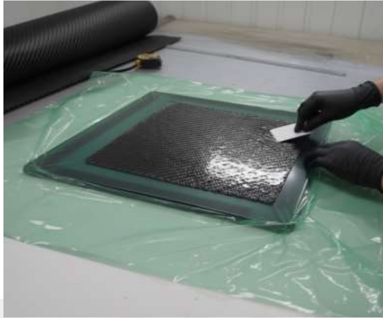
Figure 3.9. Hand lay-up process during lamination
