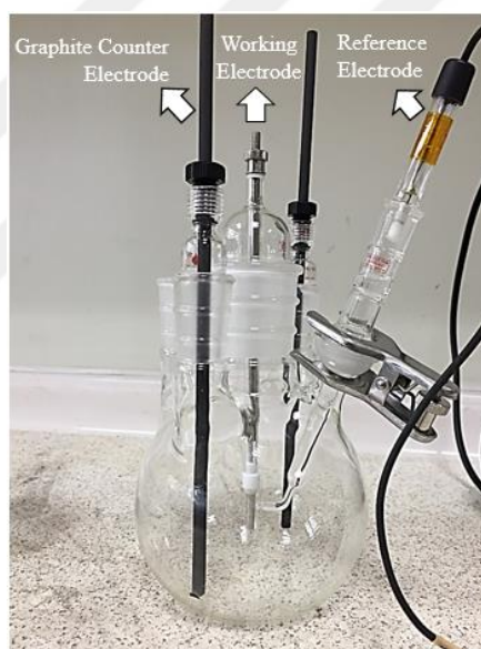
Figure 3.6. The electrochemical cell containing three electrodes.
