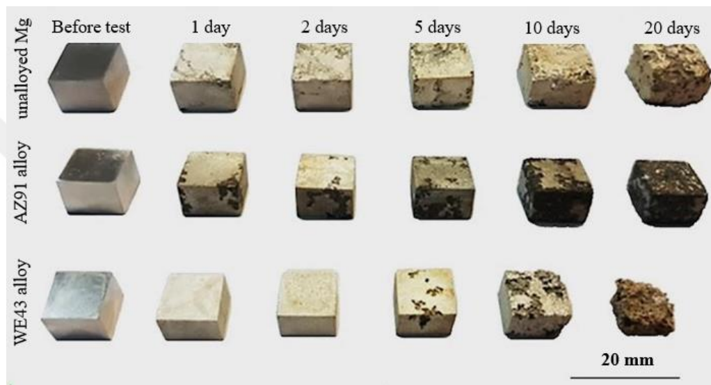
Figure 4.60. Macro-structural changes of Mg/Mg-alloys after immersion in SBF.
