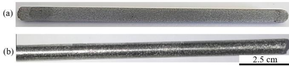
Figure 4.22. Macro images of (a) porous Ti6Al4V alloy rod and (b) manufactured Ti6Al4V-Mg composite rod.
