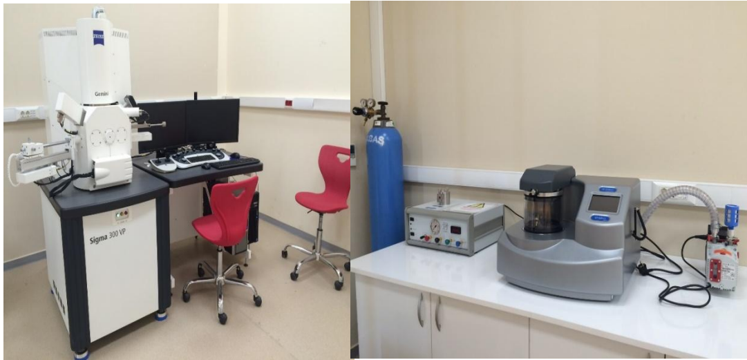
Figure 5.35 Carl Zeiss 300VP SEM and QUORUM Q150 RES device (IKCU merkeziarařtırmalab, 2020)
