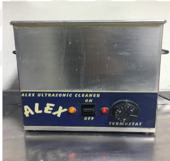
Figure 3.11. Cleaning of specimens in the ultrasonic bath
