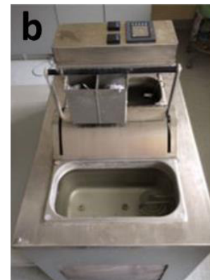
Figure 3.15.a. Subgroups to be subjected to thermocycling, and b. Bath of the thermal cycler
