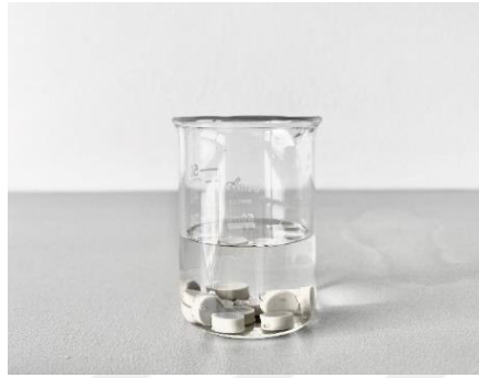
Figure 3.4. Rinsing of specimens in de-ionized water
