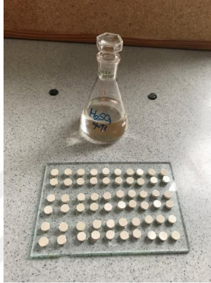
Figure 3.6. Etching of PEEK specimens with 98% Sulfuric acid.
