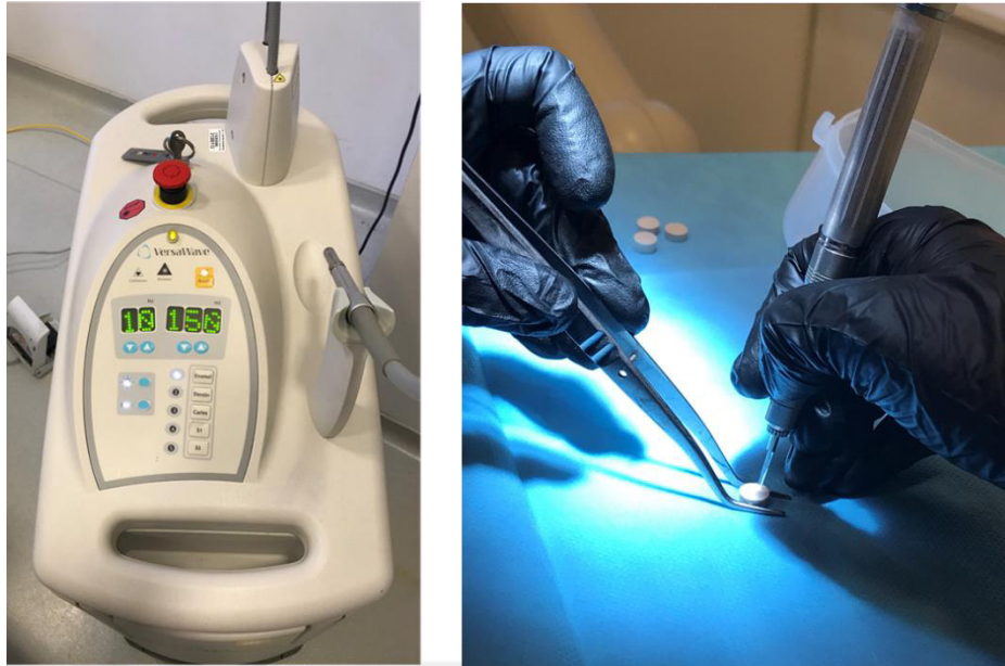
Figure 3.7.a. Er:YAG laser device (Er: YAG laser, Hoya ConBio, Fremont, USA) b. Er:YAG laser application on surface of the PEEK specimens
