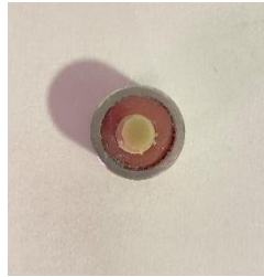
Figure 3.16. Specimen embedded in self-curing acrylic resin
