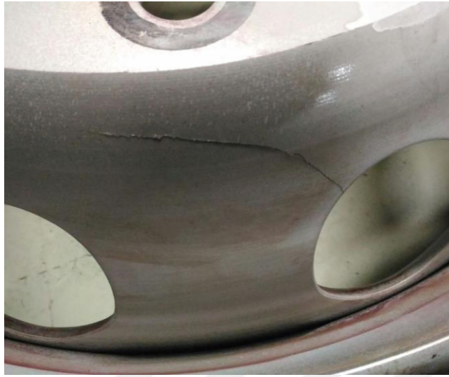
Figure 5.7 Wheel fatigue failure picture (Personal archive, 2020)
