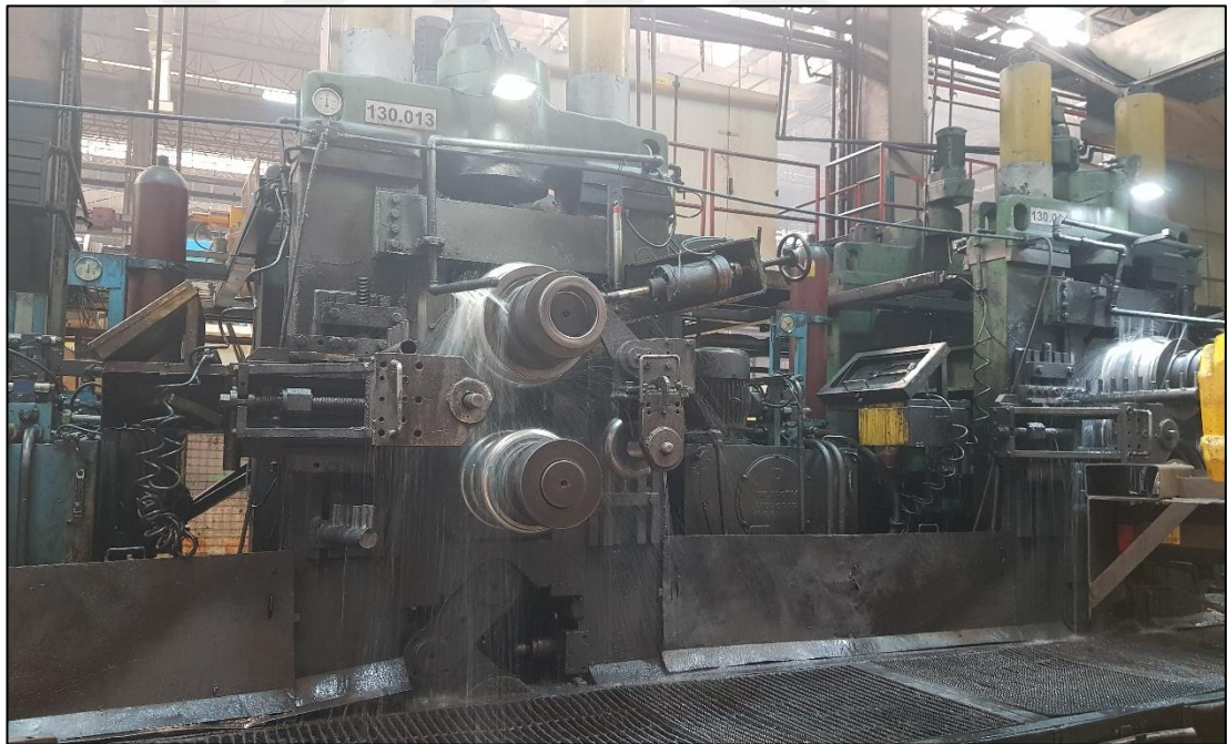
Figure 2.1 Rim flow forming process (Personal archive, 2020)
