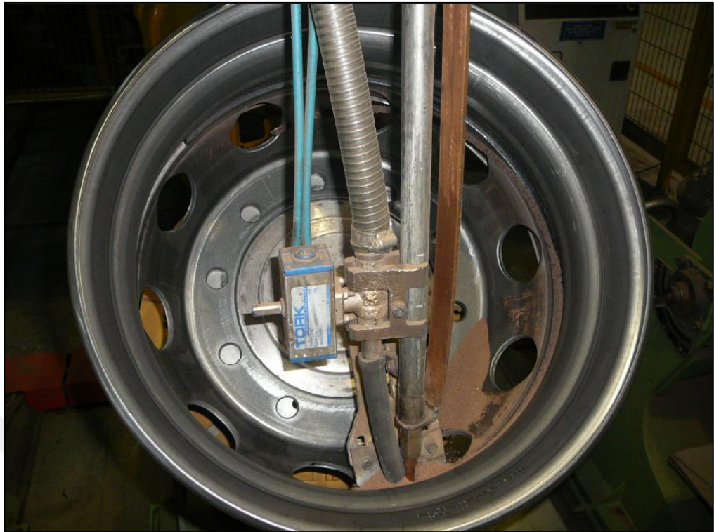
Figure 2.7 Wheel assembly welding process (Personal archive, 2020)
