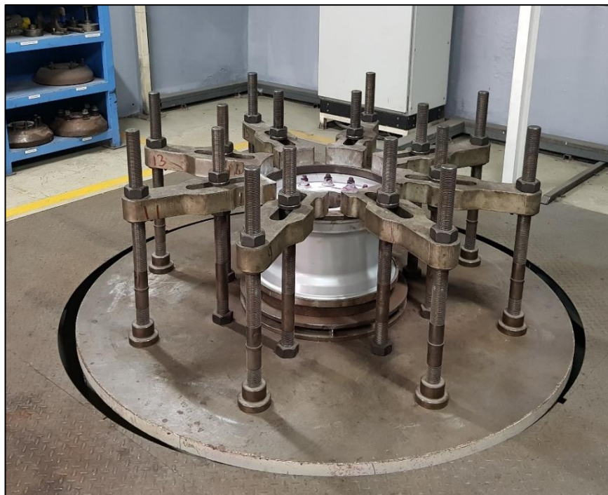
Figure 4.4 Cornering fatigue test machine (Personal archive, 2020)
