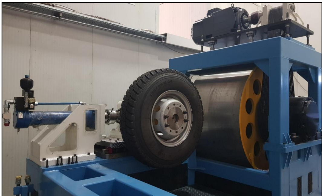
Figure 4.2 Radial fatigue test machine (Personal archive, 2020)
