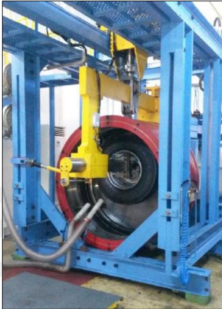
Figure 4.6 Biaxial fatigue test machine (Personal archive, 2020)
