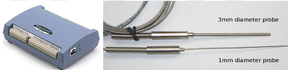
Figure 3.18. Measurement devices; data logger (left), K-type thermocouples (right)
