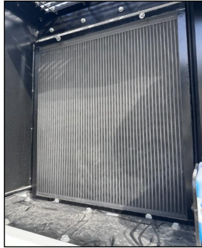
Figure 15: Radiator that is used in excavator
