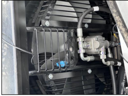
Figure 16: Hydraulic Fan that is used in excavator
