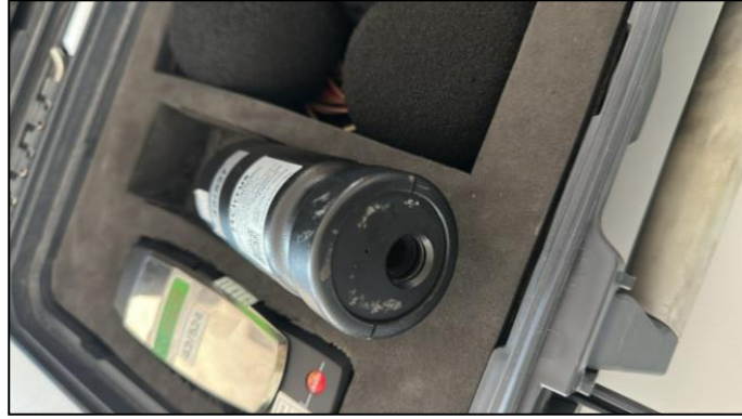
Figure 34: Sound calibrator for microphone sensitivity at 94 dBA reference.
