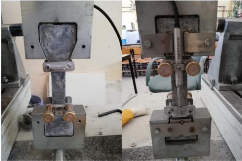
Figure 3.4 Tensile loading of bone-shaped samples (Personal archive, 2019)
