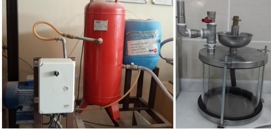
Figure 3.8 Vacuum assembly and epoxy soak chamber (Tubitak, 2020)
