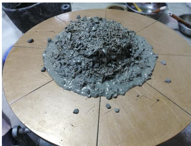
Figure 4.31 The 13 mm fiber locking of normal mortar mixtures
