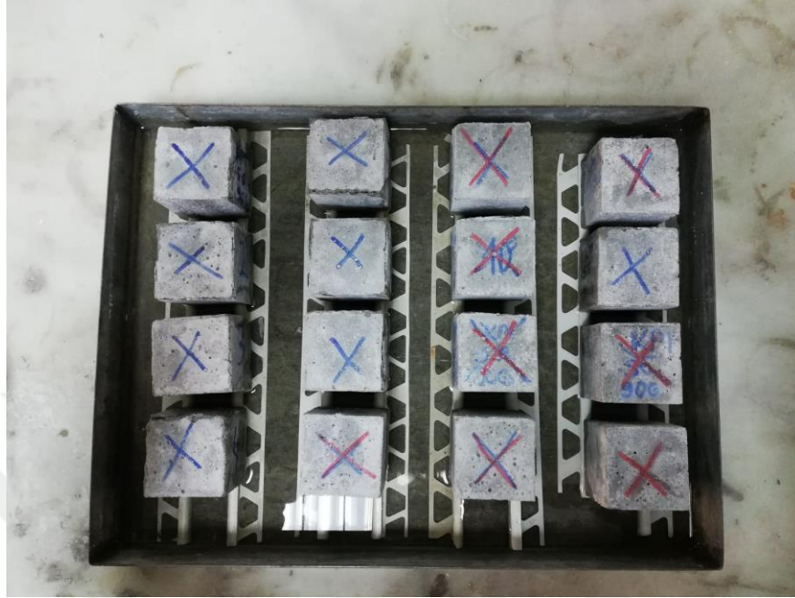
Figure 3.5 CWA test of preloaded samples (Personal archive, 2019)
