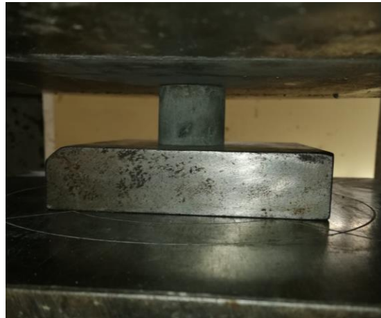
Figure 3.7 Compressive strength test of cylindrical samples (Personal archive, 2019)
