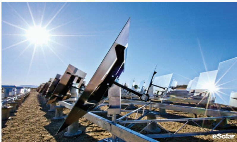
Figure 4.15 Heliostats developed by eSolar [124].
