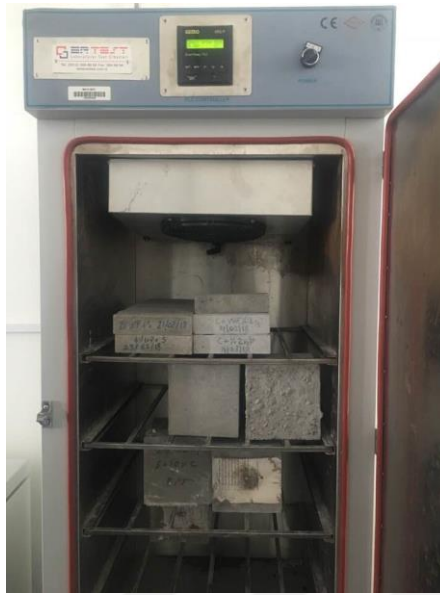
Figure 4.4: Freeze and thaw chamber
