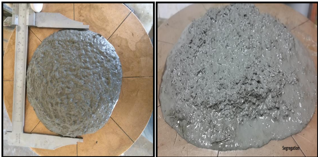
Figure 3.3 Consistency and workability of mixture (Personal archive, 2016)
