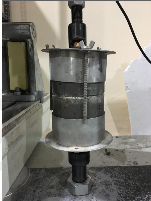
Figure 2.9 Self bonding test (Personal archive 2016)
