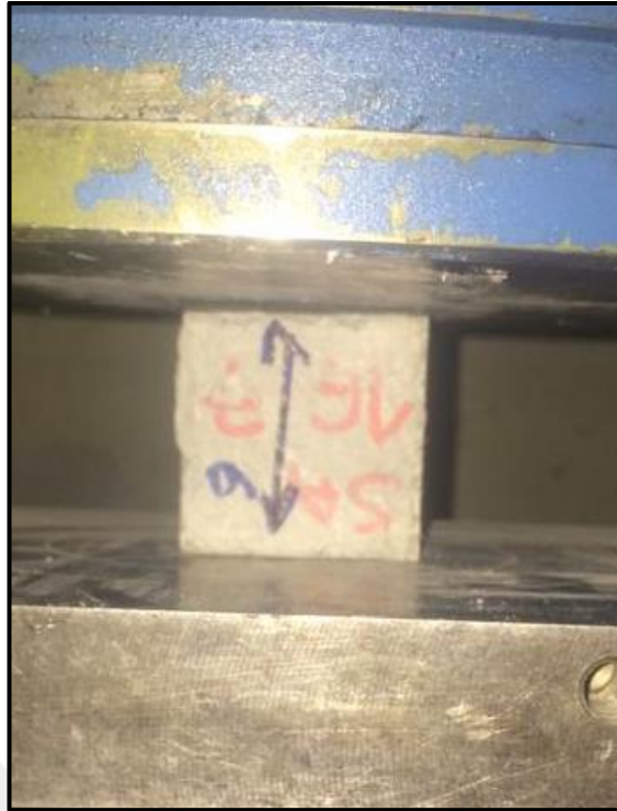
Figure 2.2 Mentioned that test must be applied on the same direction of specimens before and after healing (Personal archive, 2017)
