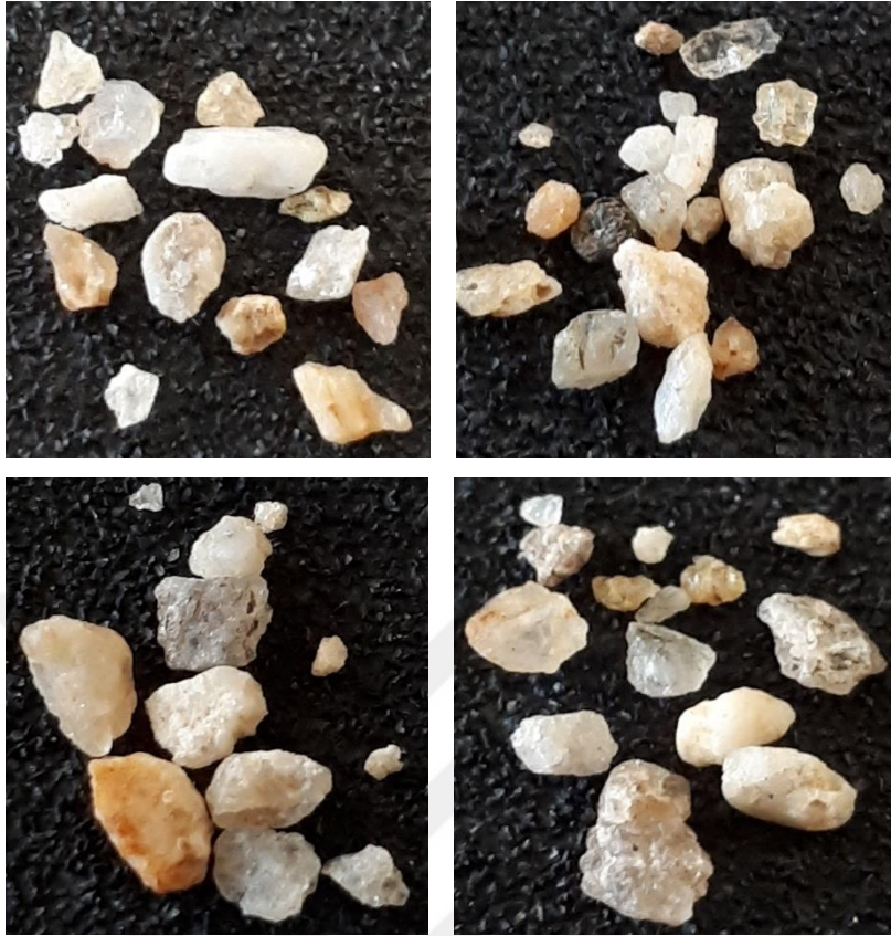
Figure 3.2. Grain shapes of Çine sand
