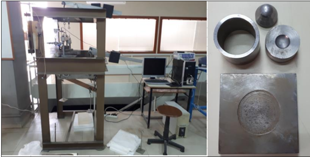
Figure 3.11. Oedometer test setup and apparatus
