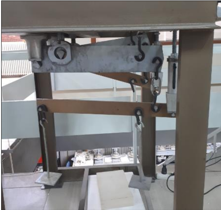
Figure 3.12. Load arms of the test system
