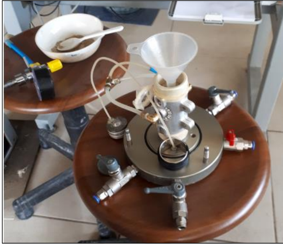
Figure 3.5. Tapped funnel deposition method
