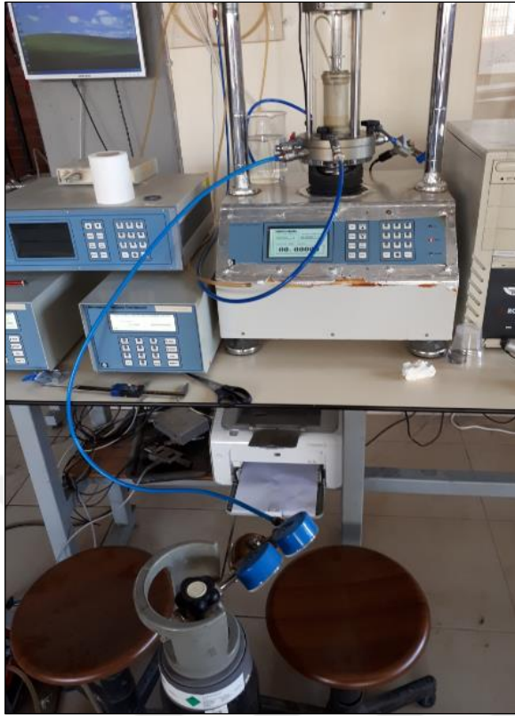
Figure 3.8. Passing CO 2 through the sample
