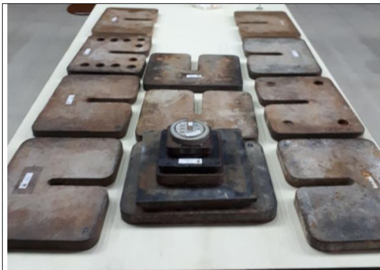
Figure 3.13. Weights used for oedometer tests
