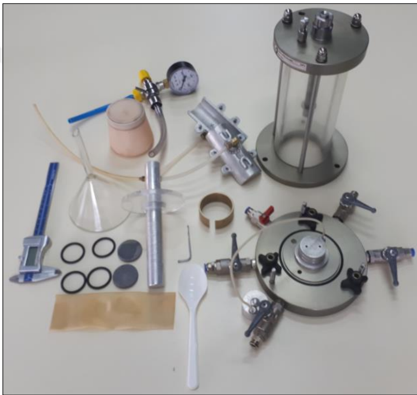
Figure 3.4. Apparatus used in triaxial tests
