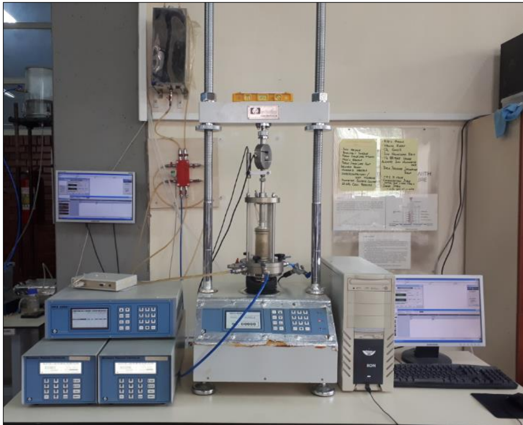
Figure 3.3. VJ TECH automated triaxial test system
