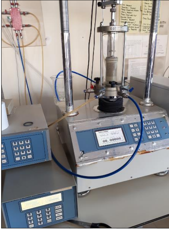
Figure 3.9. Percolation of de-aerated water
