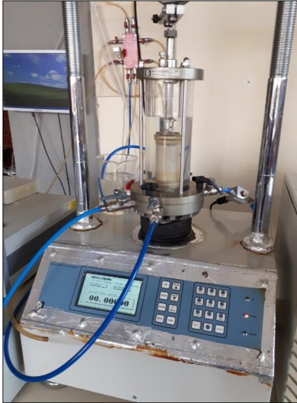
Figure 3.7. Filling the cell with water
