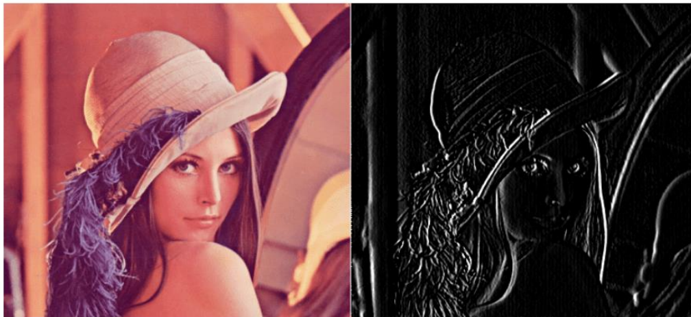
Figure 2.12 An image convolved with vertical Sobel filter
