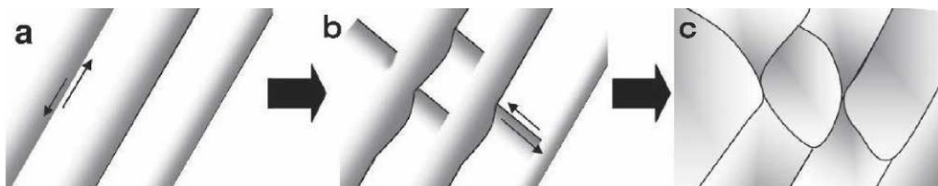
Figure 2.17 Subgrain (Giant fault) formation schema [11].
