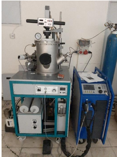
Figure 3.1 Edmund Bühler GmbH arc melting device and water-cooled copper crucible mold.
