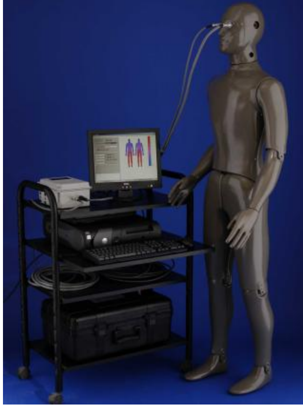
Şekil 2.2 Isıl manken Newton (Measurement Technology Northwest, 2010)
