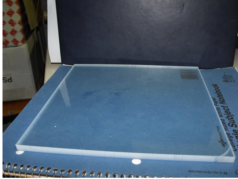
Figure 3.3: KURARAY organic scintillator 20 \times 20\text{ cm}^2 and 1.5\text{ cm} thick.
