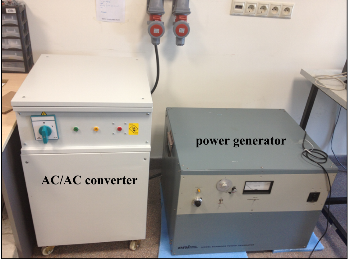
Figure 3.9: AC/AC converter and power generator.
