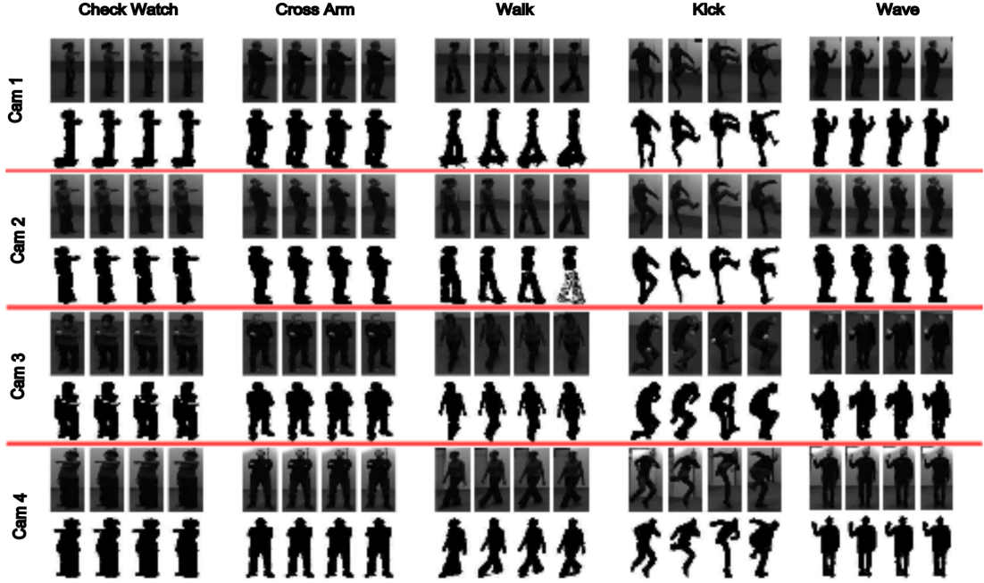
Figure 5.4: Example frames of some action classes from the IXMAS Dataset. Every actor performs every action in 3 different orientations. Cameras 1 and 2 are placed close and almost have side views. Camera 3 is installed higher than others, therefore cross camera recognition using camera 3 is hard due to great variation in viewpoint. Camera 4 is the most controlled one having a reasonable height and side view. In cropped images, it is shown that true body pose gets lost in some views depending on the camera and actor orientation. Also, background subtraction results with some defects ( median filter is applied over binary images prior to feature extraction.)
