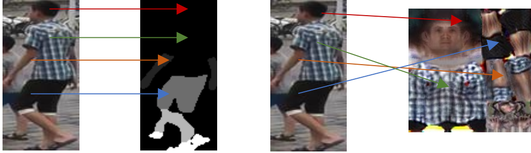
Figure 1.1: Texture estimation is not aligned, unlike many tasks with input-output alignment (e.g., part segmentation).
