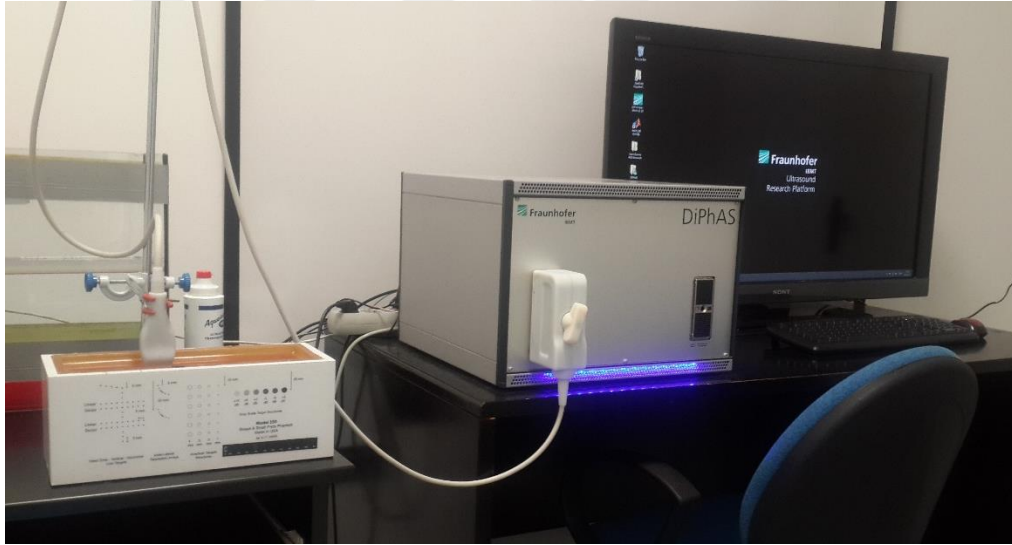
Figure 3.6: Experimental setup for phantom measurements. The setup consists of DiPhAS integrated with a personal computer, a phantom, a phased array transducer positioned on top of the phantom surface, and a holder for fixing the transducer array position.
