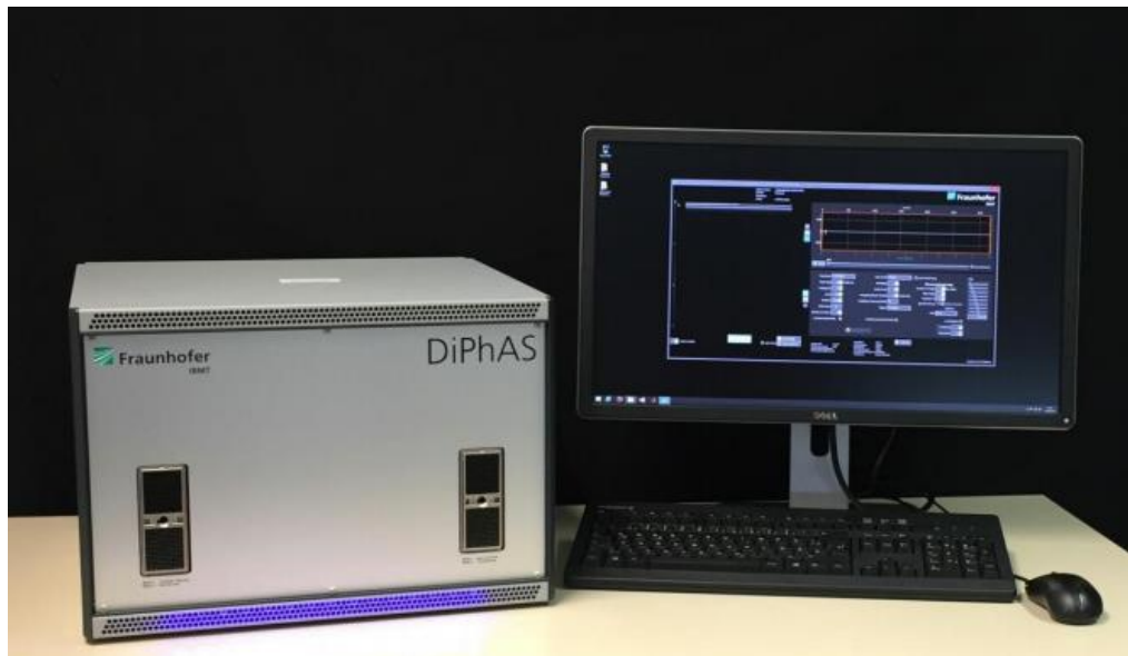
Figure 3.1: The ultrasound research scanner, Digital Phased Array System (DiPhAS), used in the measurements for ultrasound data acquisition.
