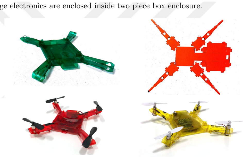
Figure 3.3: First prototype of the foldable micro quadrotor equipped with Arduino Nano, MPU6050 IMU, and coreless DC motors.
