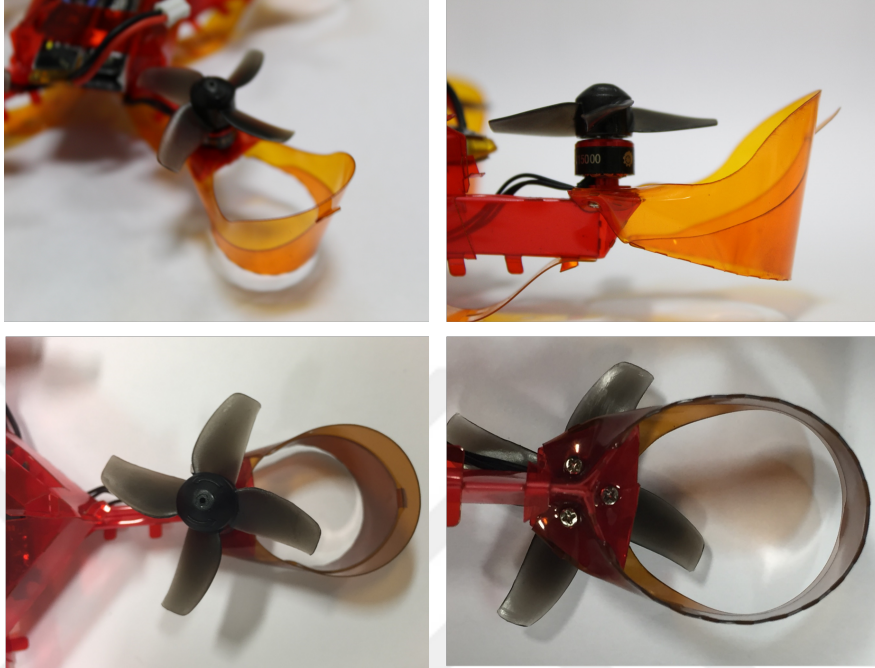
Figure 3.9: Implementation of the bumper, mounting point and half-fold is visible.
