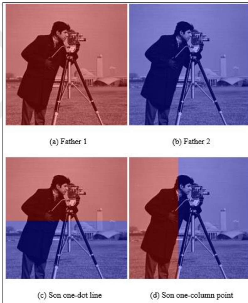
Figure 3.10: Examples of one-point row and column crossover operators.
