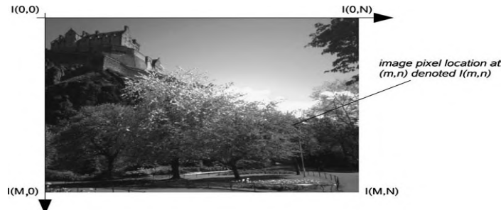
Figure 1: 2-D Cartesian Coordinates Space of an M X N Digital Image [2] .
