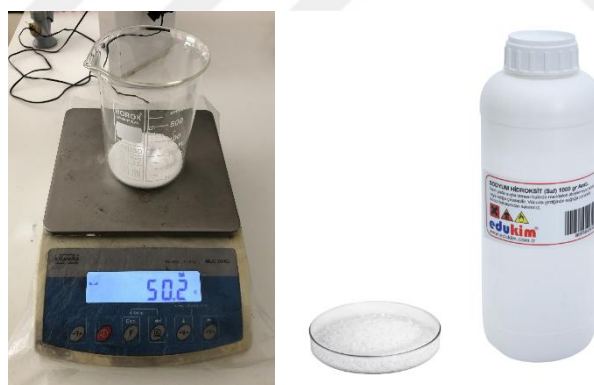
Figure 3.18. Granulated sodium hydroxide is used as an electrolyte
