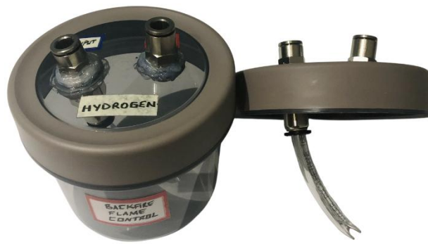
Figure 3.13. Backfire flame control equipment
