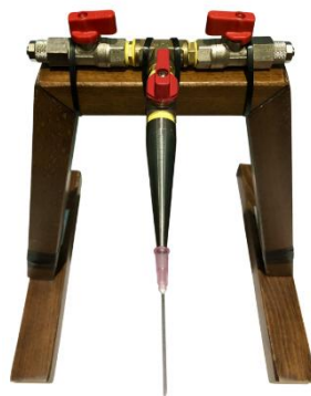
Figure 3.14. Special design T-burner with needle tip on the platform
