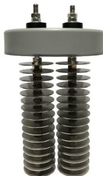
Figure 3.16. Probes used as anode and cathode
