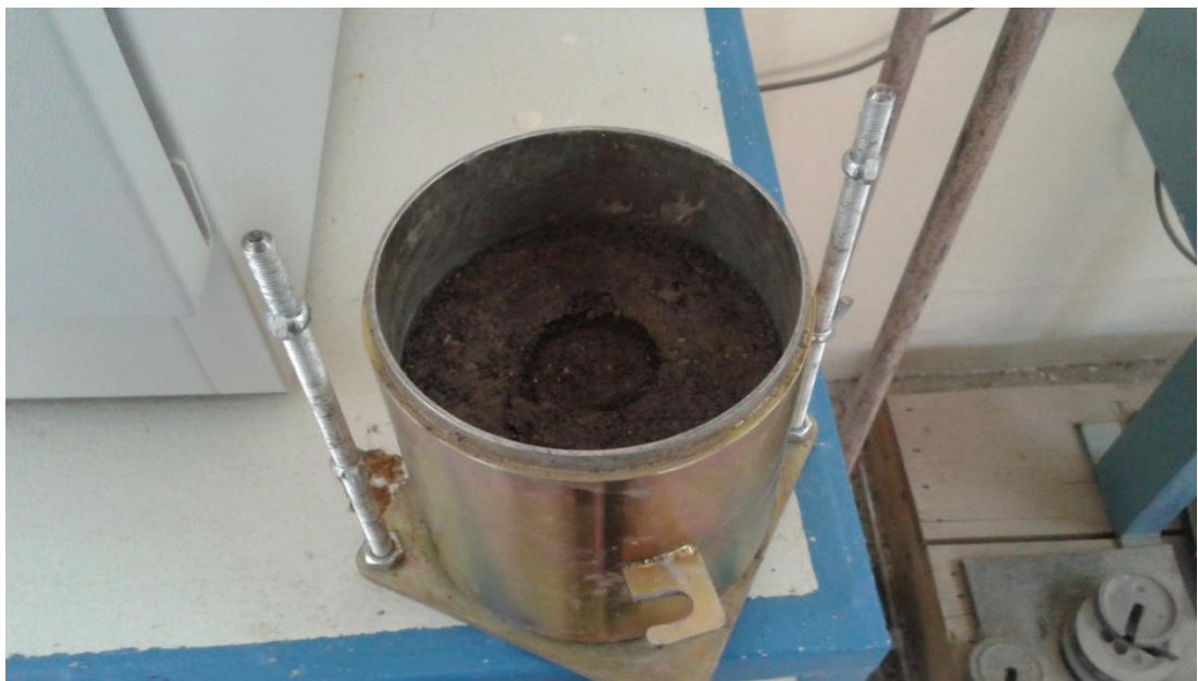
Figure A.8 Sample after the CBR test
