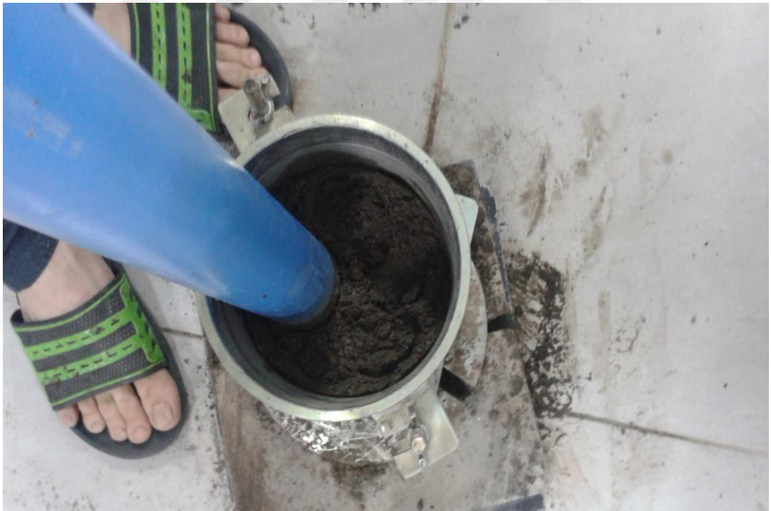
Figure A.4 Modified compaction test
