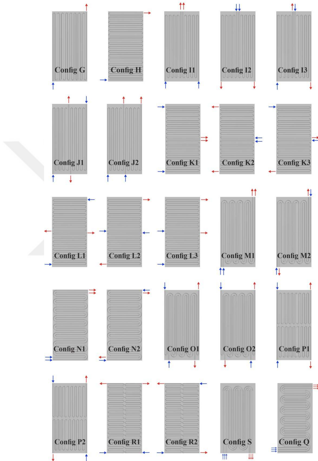
Figure 3.3. Different serpentine tube PVT collector configurations
